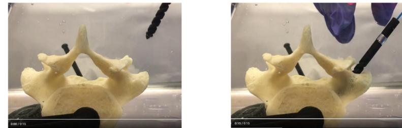
**Figure 2.** Data collection. Left: before data collection; Right: fully inserted drill tip
