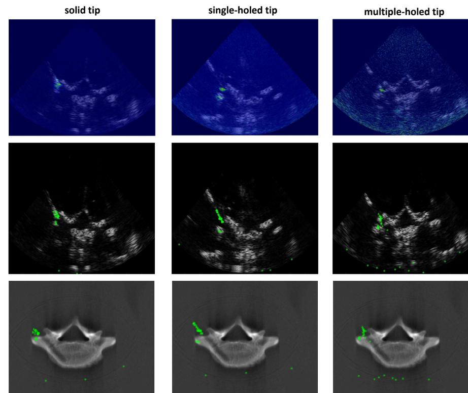
**Figure 3.** Top row: representative PA image overlaid on US image; Middle row: tracking results on US image; Bottom row: coordinates overlaid on CT registered image.
