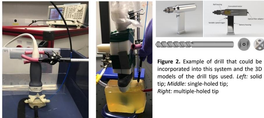
**Figure 1.** Data collection. A) phased array set-up for drill tracking experiments B) linear array set-up for blood visualization
