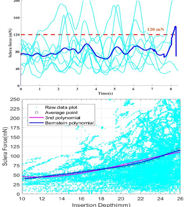
5 trials/experiment and switching target in random order. The insertion depth and forces were measured by the force-sensing tool and recorded.
