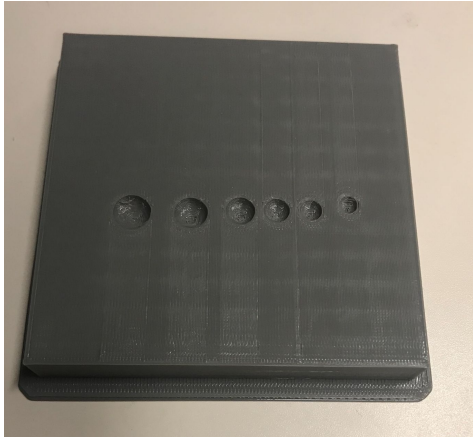
Figure 2. The image above depicts the pivot calibration holder we used to conduct our pivot calibration. The multiple holes were printed as we did not originally know the best size for our tool.
