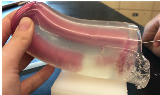
Fig. 7. The resulting first prototype with a vaginal cavity, a rectum (both in pink), and a less visible cervix (transparent) under needle insertion.
