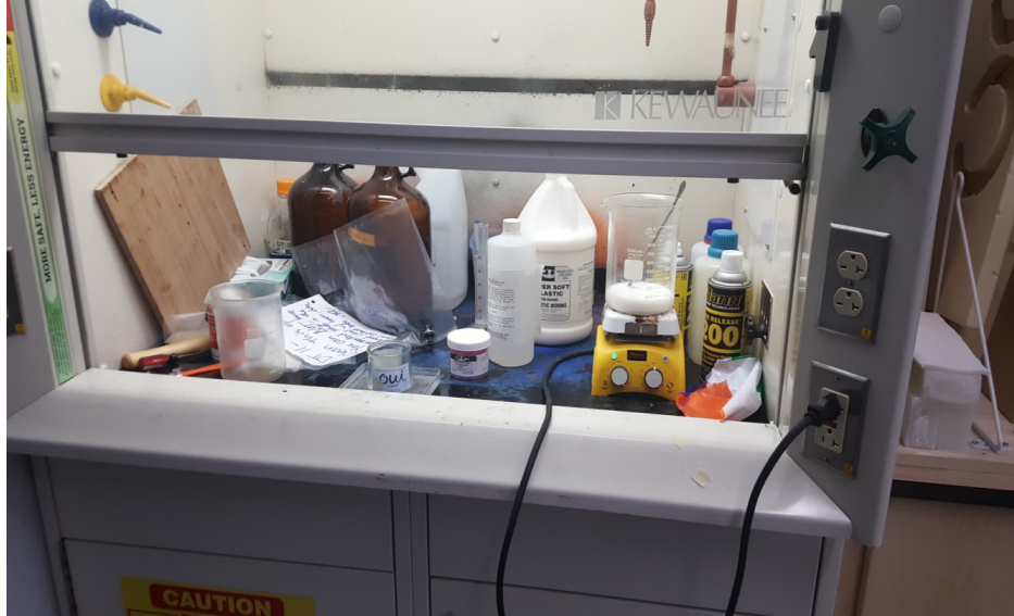
Fig. 3. Image of sample plastisol heating and curing environment showing hood, plastisol, dyes, glass molds and a heat plate.
