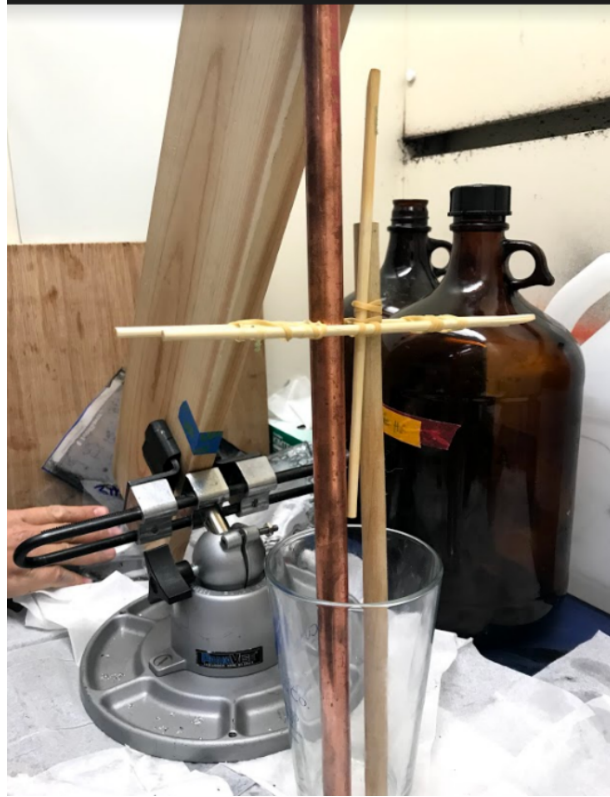
Fig. 4. Molds used in the manufacturing of the phantom were fastened in order to maintain the shape of the cavities in a glass container.
