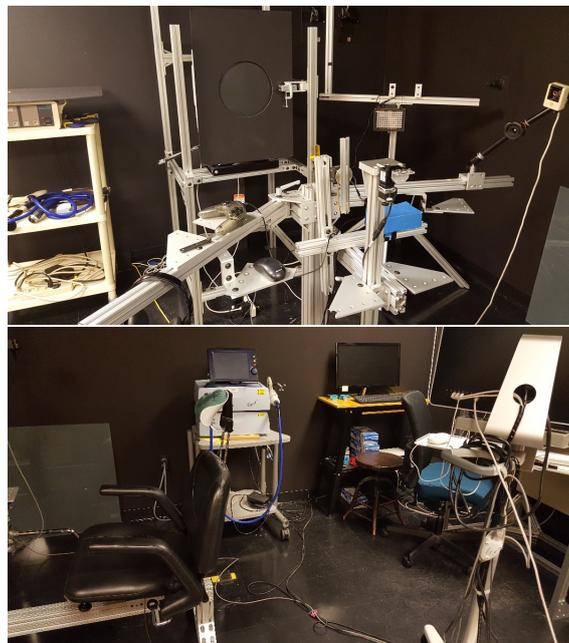
Figure 3: Above: An illustration of the bite bar setup where subjective visual vertical was assessed. Below: The subject's chair and the TMS coil station set up in the background.
