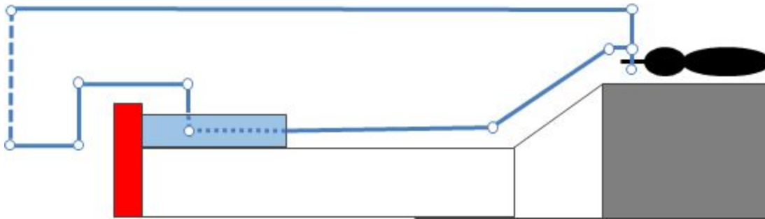
Figure 22. Robot path with the integrated robot and automated dissector system using the keypoint vision algorithm. All of the image processing is done from an overhead camera, and thus a less complicated path is needed to pick up the mosquito, though the difference in stage-to-cartridge height has to be accommodated for.
