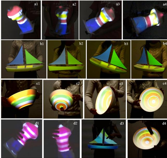
**Figure 10.** Real projection mapping effect of Pmomo. The white plastic models in the pictures are shaded with colorful textures by projection. All the pictures are video snapshots of projection effect on moving objects.
