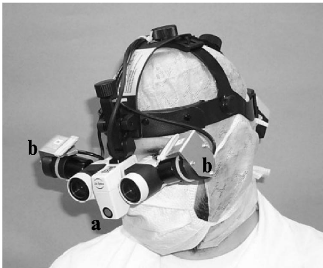
Fig. 2. A photograph of the prototype of the Varioscope AR. Visible are (a) the base instrument and (b) the housing for the projection optics with the miniature displays. Since the Varioscope AR is designed for stereoscopic vision, two display systems are connected to the Varioscope AR.
