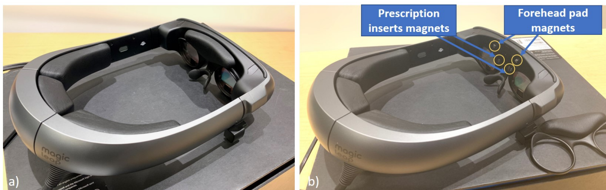
Figure 2.1: a) Magic Leap One headset with forehead pad and an empty prescription insert that comes with the box. b) 4 magnets that connect the customizable components to the headset
