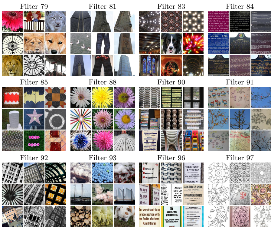
Fig. 7: Top 9 activated images from a random subset of 10 millions images from YFCC100M for the 100 first filters in the last convolutional layer of an AlexNet trained with DeepCluster (we do not display humans).
