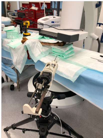
Figure 6: Experiment setup of femur cement injection using the nView system.
