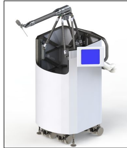
Figure 2: Full CAD assembly of the Galen Mk. 2 platform [3]
