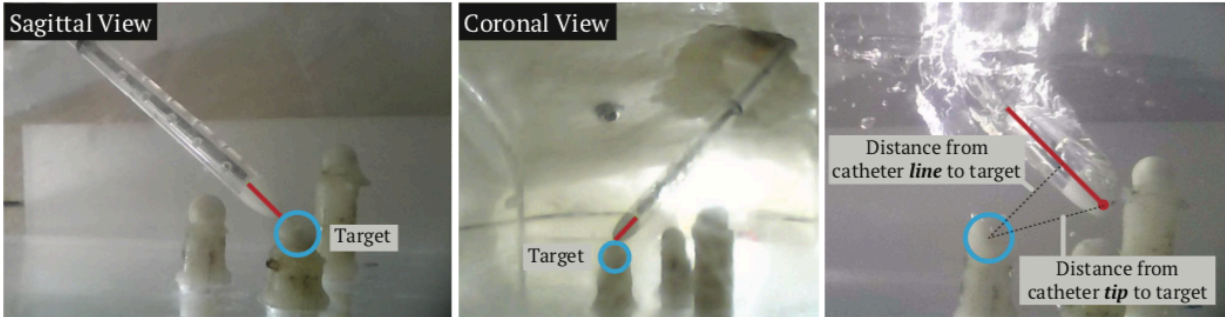
Figure 4: Visual description of the two task accuracy measures. Left two photos show the definition of “distance between catheter tip and target.” Right photo shows the definition of “distance from catheter line to target.”
