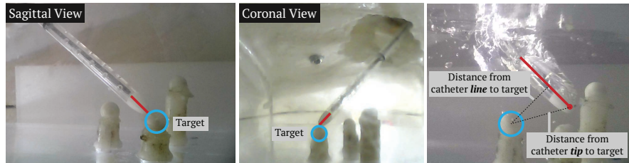
Fig. 6: Left: Sample images from two borescope cameras, showing measurements. Right: Distances from the target to the catheter tip and catheter direction
