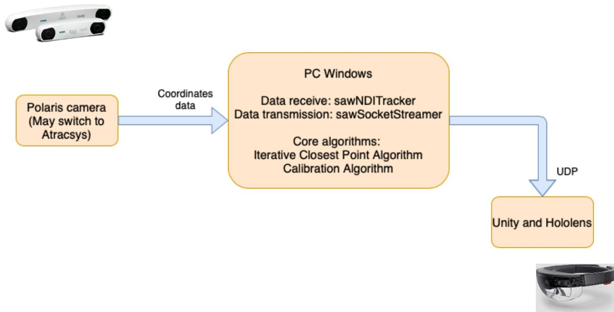
Figure 4. The proposed preliminary system components.
