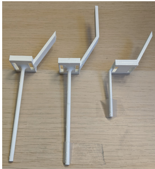
Figure 2.3. Calibration object augmented design. Left to right: design iterations.
