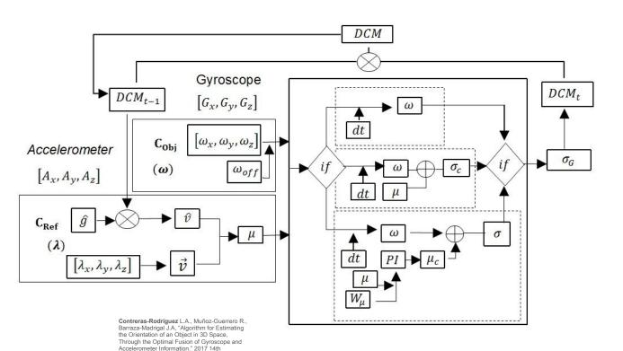
$_{\odot}$  - Gyroscope data alone with offset correction  $\sigma_{\rm C}$ - Plain estimation including gyroscope data and accelerometer data  $\sigma$  - Estimating using a PI feedback controller to remove drift and reduce noise (includes gyro + accelerometer data)
