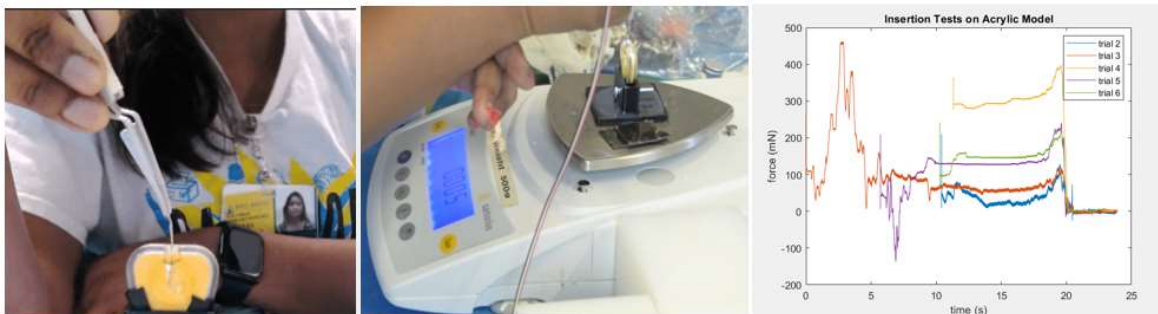
Figure 7. From left, electrode insertion test with plastic cochlea model, scale readings measured underneath, and analyzed data using MATLAB
