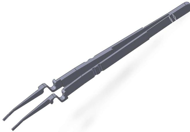
Figure 2. Prior 1 DOF force-sensing forceps model
