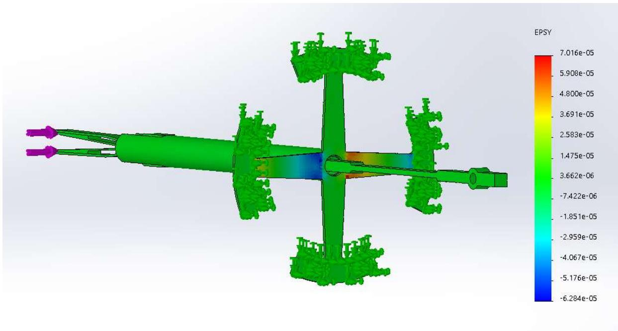
Figure 10. Strain result from lateral force (x)
