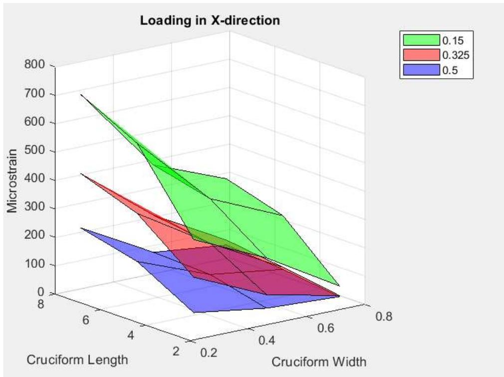
Figure 7. Cruciform strain at various length, width, and thickness
