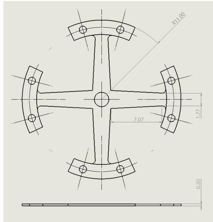
Figure 8. Important geometries of the cruciform
