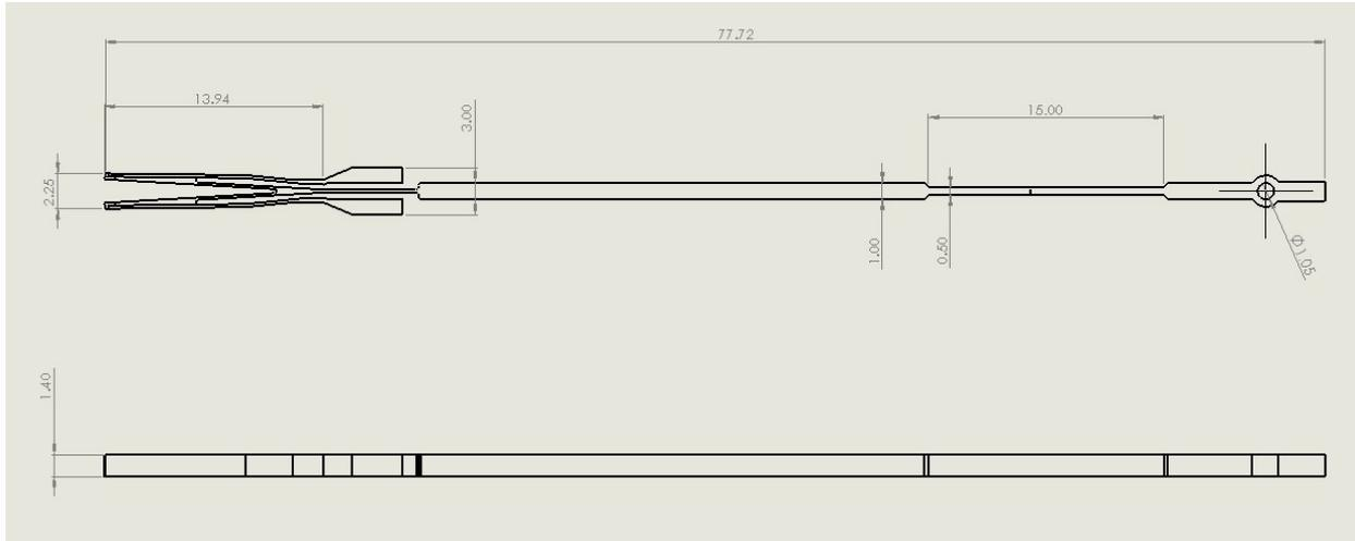
Figure 6. Important geometries of the jaw portion
