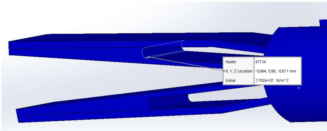
Figure 7. Force concentration during actuation
