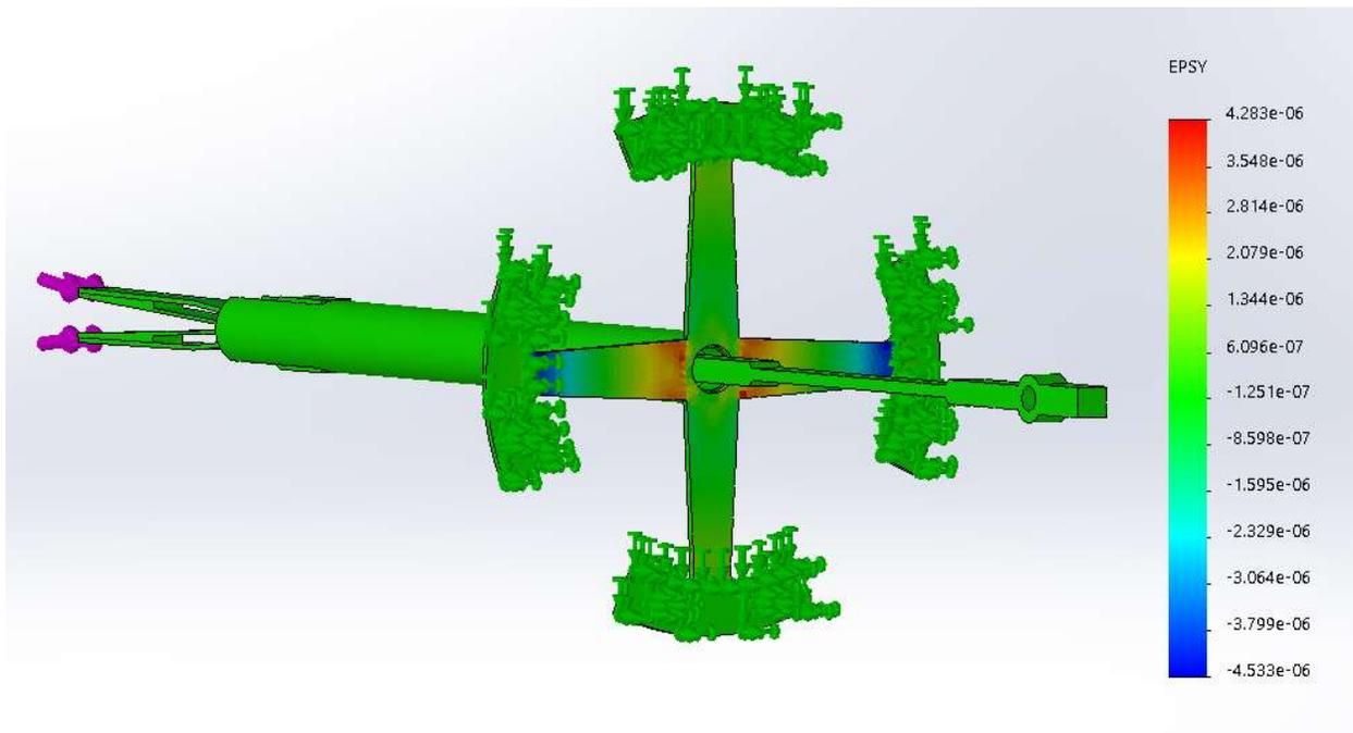
Figure 12. Strain result from axial force (z)
