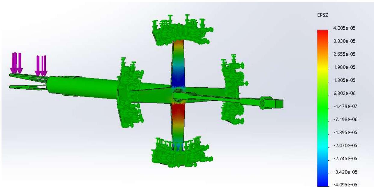
Figure 11. Strain result from lateral force (y)
