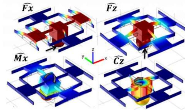
Figure 6. MEMS 6 DOF force measurement cruciform design
