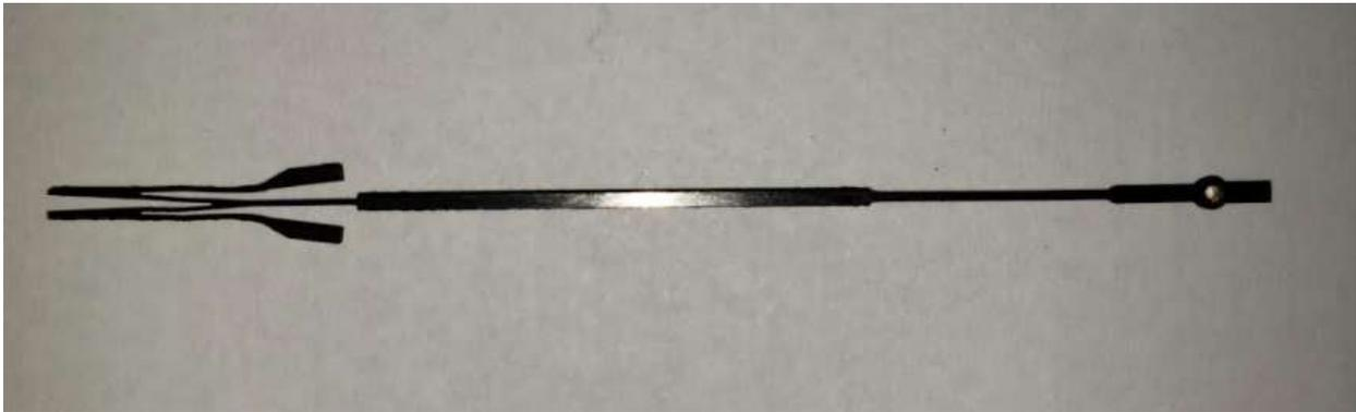
Figure 14. Prototyped jaw and middle rod
