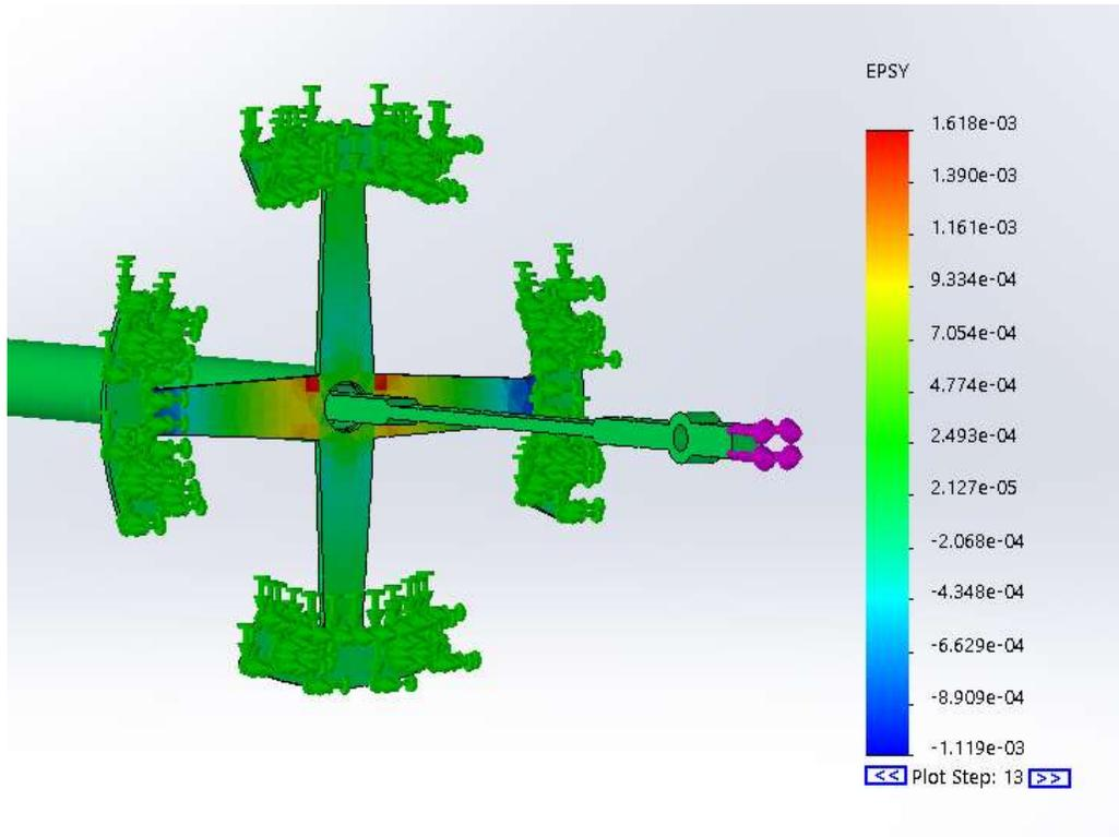
Figure 9. Strain result from actuation alone
