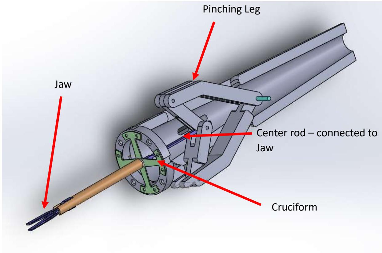
Figure 5. Final CAD model of the forceps
