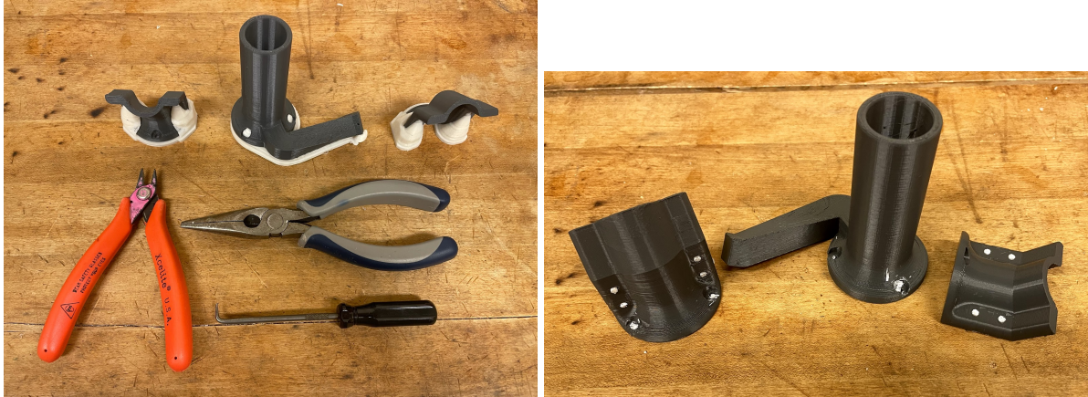
Figure 9: Tools used to remove support material and final result.
