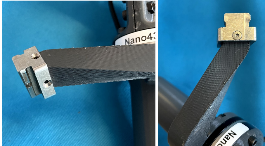
Figure 13: Attaching the adapter to the grip.
