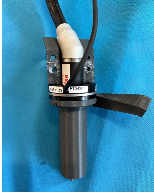
Figure 11: Intermediate assembly step with drill placed in half-assembled device.
