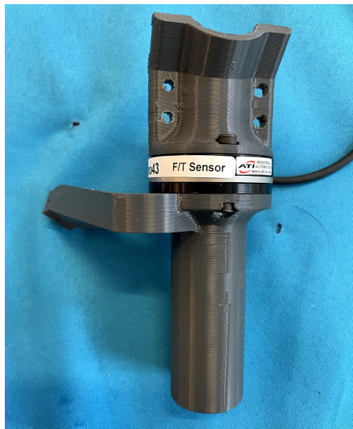
Figure 10: Assembling the grip and first half of the clamp onto the sensor.
