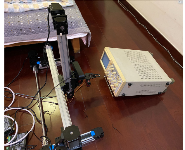
Fig 1. Overall structure of end-effector interacting with oscilloscope
