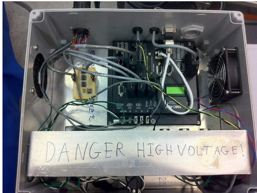
Figure 9: Electronics enclosure interior. Note: High voltage (120V) warning is for maintenance safety. System is fully grounded and enclosure is closed during normal use.
