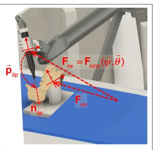
Figure 3: Robotic Cutting
