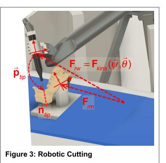
We wish to use the hand-over-hand surgical robot shown in Figure 3 to assist in performing the cuts. Here, the position of the robot's tool holder relative to its base is  $\mathbf{F}_{rw}(\vec{\theta}) = \mathbf{F}_{kins}(\vec{\psi},\vec{\theta})$ , where  $\vec{\psi}$  are structural parameters associated with the robot design, and  $\vec{\theta}$  are the positions of the joints of the robot. The robot controller is also able to compute the Jacobean
