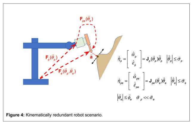
Consider the kinematically redundant robot shown in **Error! Reference source not found.** The robot has a moderately slow, but very strong and precise proximal robot and a much faster fine positioning robot carrying a surgical tool. The pose of the tool's coordinate system is given by
