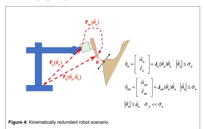
Consider the kinematically redundant robot shown in Figure 4Error! Reference source not found.. The robot has a moderately slow, but very strong and precise proximal robot and a much faster fine positioning robot carrying a surgical tool. The pose of the tool's coordinate system is given by
