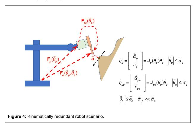
Consider the kinematically redundant robot shown in Figure 4. The robot has a moderately slow, but very strong and precise proximal robot and a much faster fine positioning robot carrying a surgical tool. The pose of the tool's coordinate system is given by
