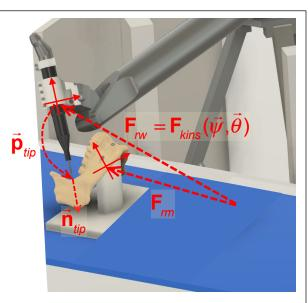
Figure 3: Robotic Cutting
